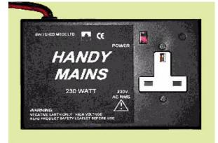
**GENERAL.** These economic power adaptors convert battery voltage to mains level voltage, for powering computers, printers, etc. The units have an output power of 250 watts short term, with surge handling up to 500 watts. Continuous available power, quoted as 200W, is limited automatically by case temperature.
